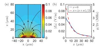
FIG. 3. (Color online) (a) Zero-point electric field distribution around superconducting CPW cavity with a center trace of 20  $\mu$ m and a 10  $\mu$ m gap. (b) Field distribution and vacuum coupling strength to the  $90s_{1/2} \rightarrow 90p_{3/2}$  transition as a function of height above the surface for both the resonator midpoint and gap center, which falls off rapidly on a length scale comparable to the slot width w.
